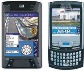
NetPDA & NetCell PTZ-enabled handheld IP video clients
