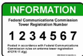
Tower Registration Sign
