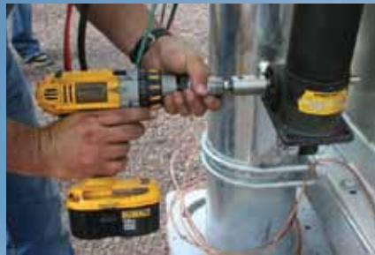
Raises and lowers using hand drill or manual hand wheel.
