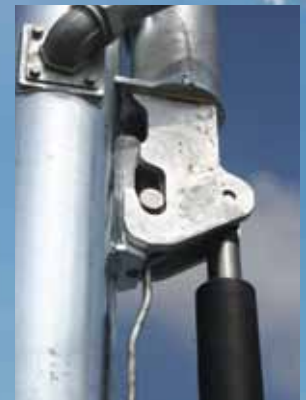
Non hydraulic jack screw with locking mast for secure operation and minimal maintenance.
