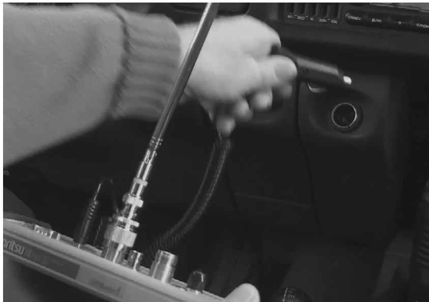
Figure 6. LMR Master can be easily set up in the field to perform P25 coverage mapping.
