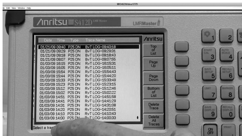
Figure 7. Traces of mapping data are automatically saved and can be later recalled and viewed from the LMR Master's front panel.
