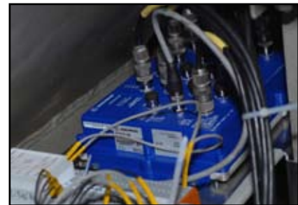
This Hirschmann OCTOPUS switch is ideal for installation in vibration-prone environments. Here, the Ethernet IP67 switch is used to provide passenger compartment video surveillance, as well as travel updates and entertainment.
