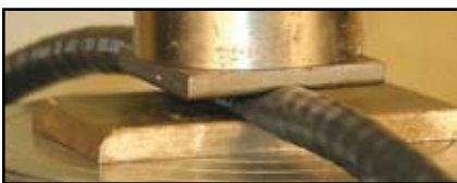
The industrial-grade armored cable fails only after a ton of crush pressure.
