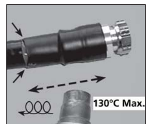
Figure 6 Shrink boot installation
